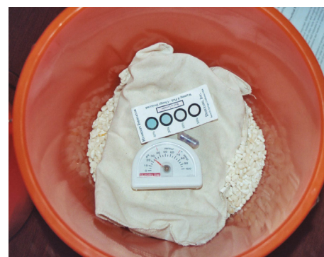
Figure 5: Using dried maize to dry a seed collection in a sealable bucket. Some low-cost relative humidity indicators have been added to monitor the moisture level inside the bucket.
