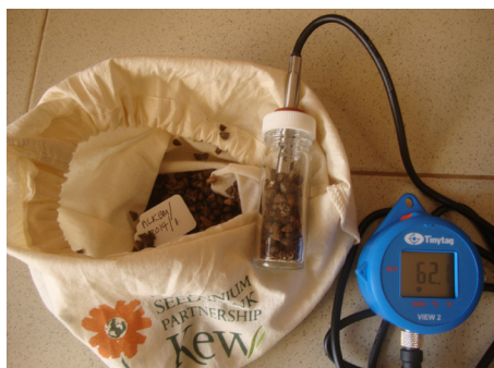
Figure 2: A hygrometer can be used in the field to measure seed eRH and ambient RH, informing post-harvest handling decisions.
