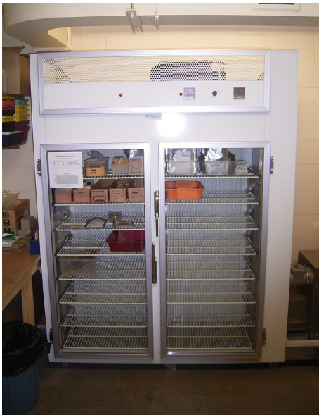
Figure 10: Bespoke drying cabinet with a dehumidification unit, at Victoria Royal Botanic Gardens, Australia.
