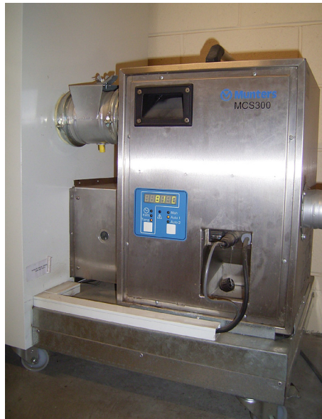
Figure 11: Dehumidification unit attached to a drying cabinet for small-scale drying.
