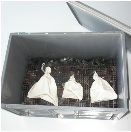
Figure 6: “Box-dryer” - plastic box with seed collections, placed above dried charcoal, on a plastic mesh.
