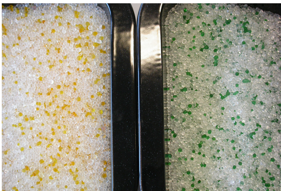
Figure 3: Methyl violet indicating silica gel beads mixed with clear silica gel, showing dry (orange) and wet (green) status
