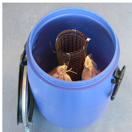
Figure 4: Sealable plastic drum containing dried silica gel, with central support from which to hang seed collections for drying.
