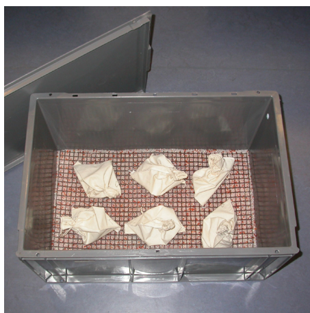
Figure 5: "Box-dryer" - plastic box with seed collections in cloth bags, placed on a plastic mesh above dried silica gel.
