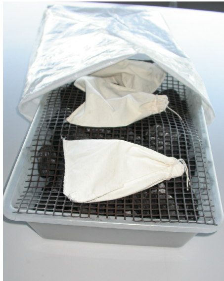
Figure 7: “Bag-dryer” - plastic sack containing a tray of dried charcoal, on which seed collections are placed on a plastic mesh.
