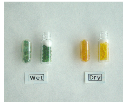
Figure 3: Loose methyl violet indicating silica gel beads, in gelatine capsules and glass vials with cotton wool.
