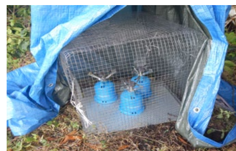
Above: Drying specimens over a gas fire. A metal cage prevents the tarpaulin getting too close to the heat source.
