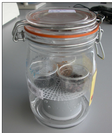
Above: Air-tight jar with lithium chloride solution, showing plastic mesh support to hold seeds above solution
