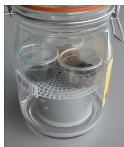
Figure 1: Air-tight jar with lithium chloride solution, showing plastic mesh support to hold seeds above solution.
