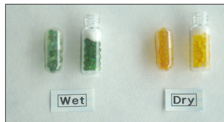
Above: Loose methyl violet indicating silica gel beads, in gelatine capsules and glass vials with cotton wool
