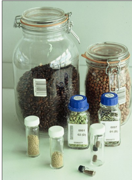
Above: Five types of glass container used at MSB - 3000cm 3 storage jar, 1000cm 3 storage jar, 100cm 3 square bottle, 30cm 3 universal bottle and 2cm 3 vial
