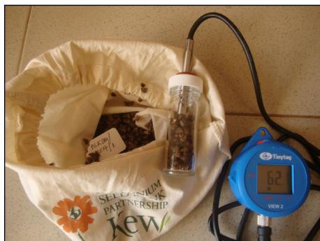
Left: A data logger used with a probe to measure seed eRH within a sealed container
