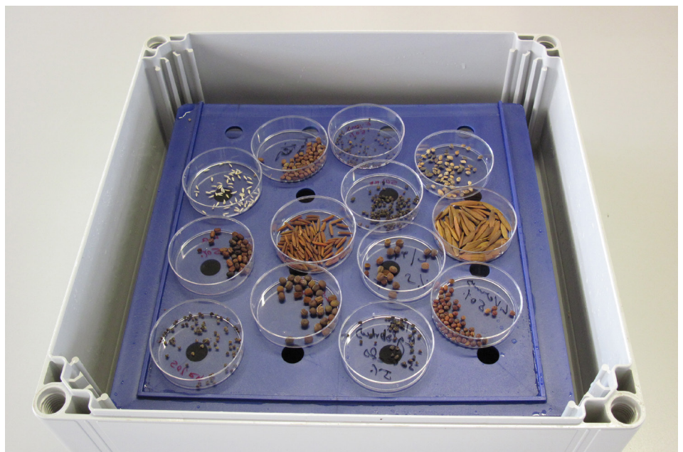
Figure 2: Plastic box with an air-tight seal, containing seed samples held above a non-saturated LiCl solution.
